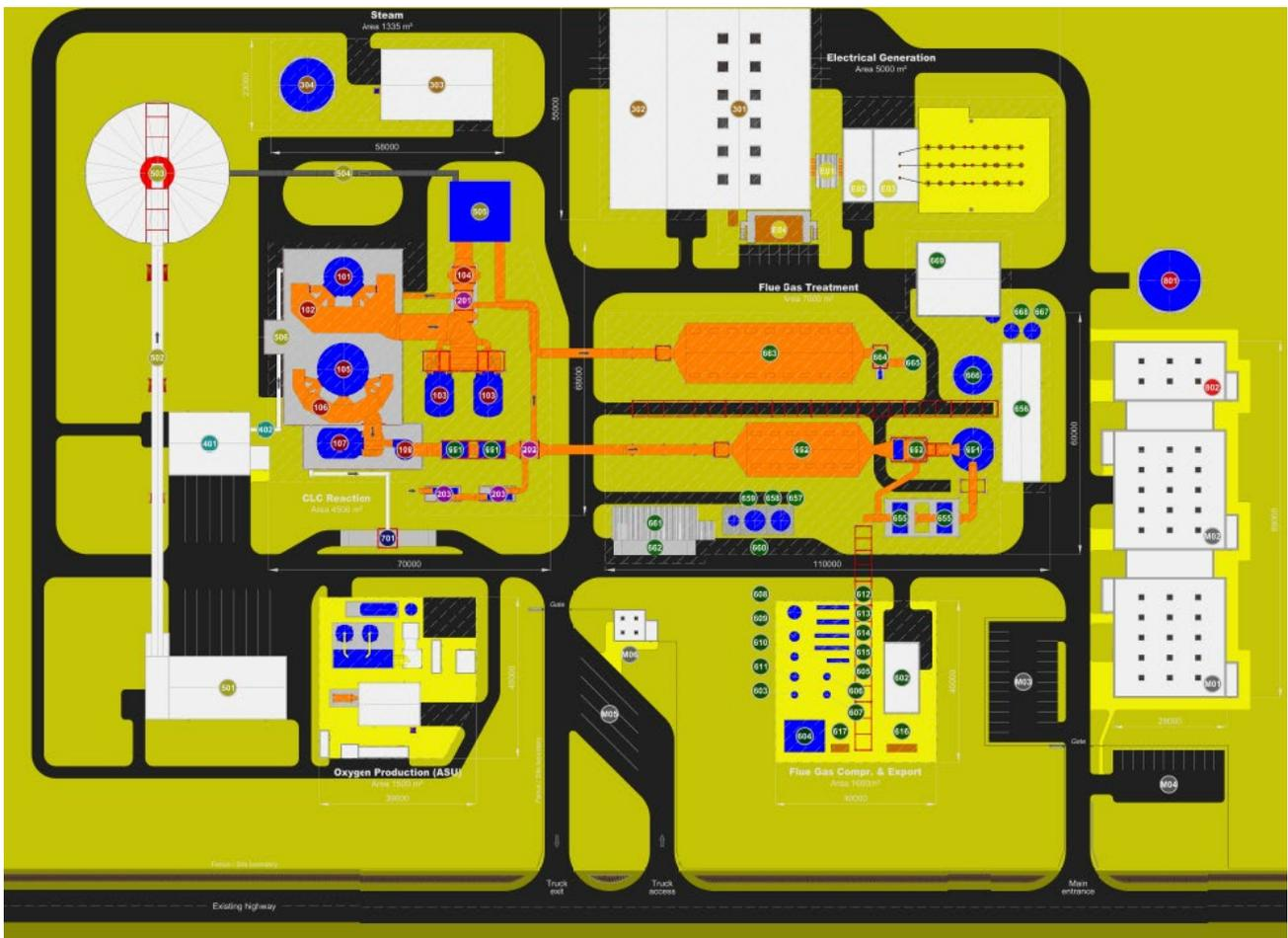
Figure 4-2: Equipment list of the CLC plant
