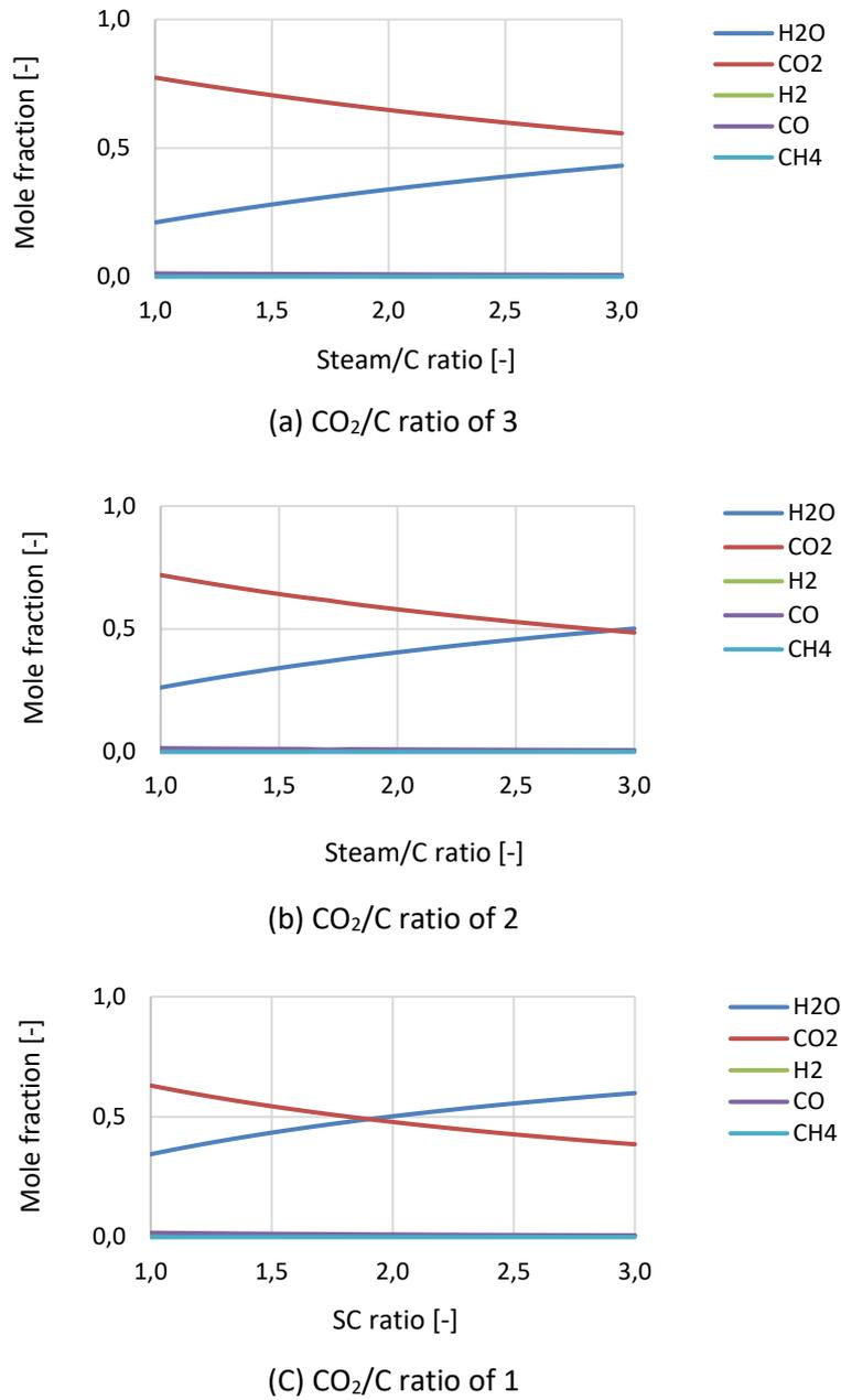
Figure 6-8 Effect of Steam/C ratio on CLC using ilmenite with different CO<sub>2</sub>/C ratios at OC/C ratio of 2 and 950 °C.
