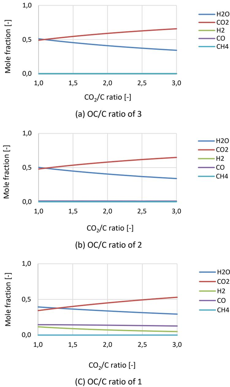
Figure 4-10 Effect of  $\text{CO}_2/\text{C}$  ratio on CLC using CuO with different OC/C ratios at Steam/C ratio of 2 and 950 °C.
