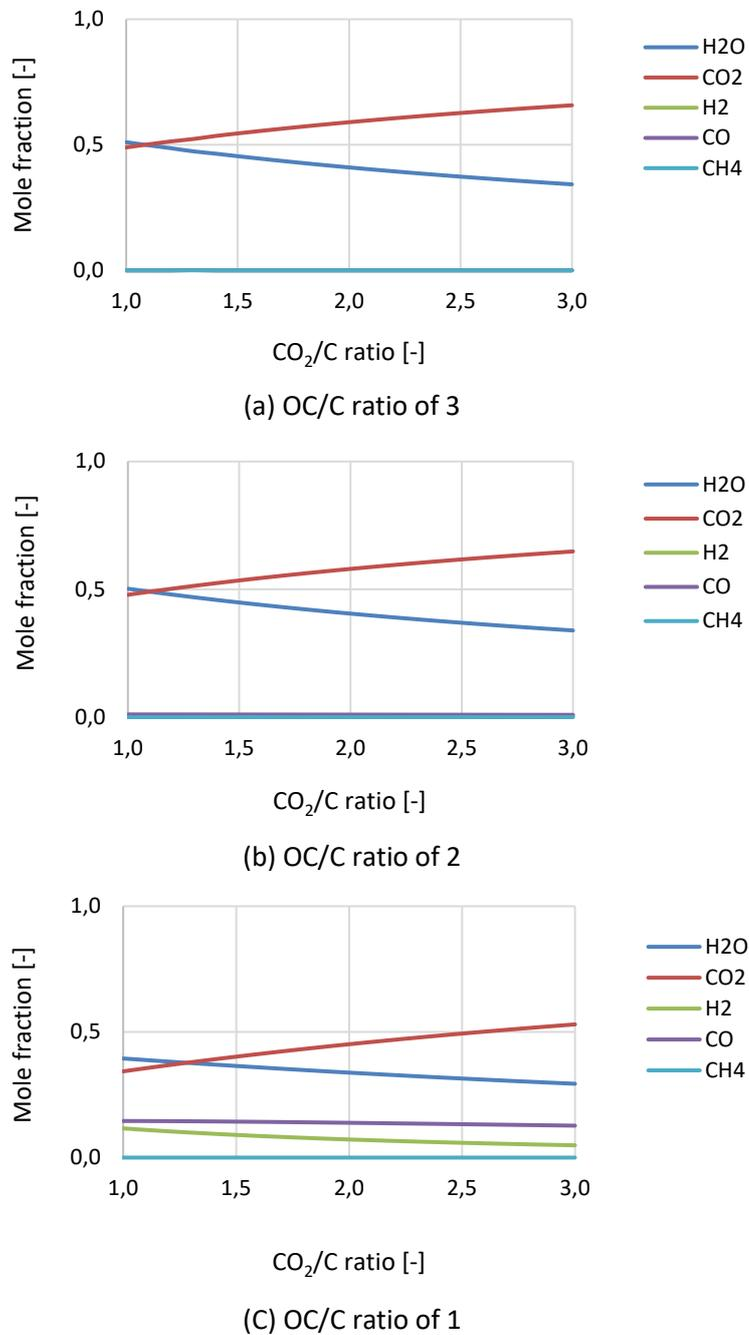
Figure 6-1 Effect of CO<sub>2</sub>/C ratio on CLC using NiO with different OC/C ratios at Steam/C ratio of 2 and 950 °C.
