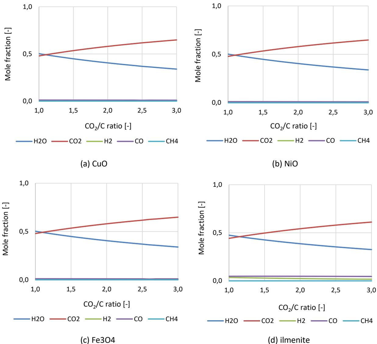
Figure 4-9 Effect of CO<sub>2</sub>/C ratio on CLC using different oxygen carriers at OC/C ratio of 2 (6 for Fe<sub>2</sub>O<sub>3</sub>), Steam/C ratio of 2, and 950 °C.
