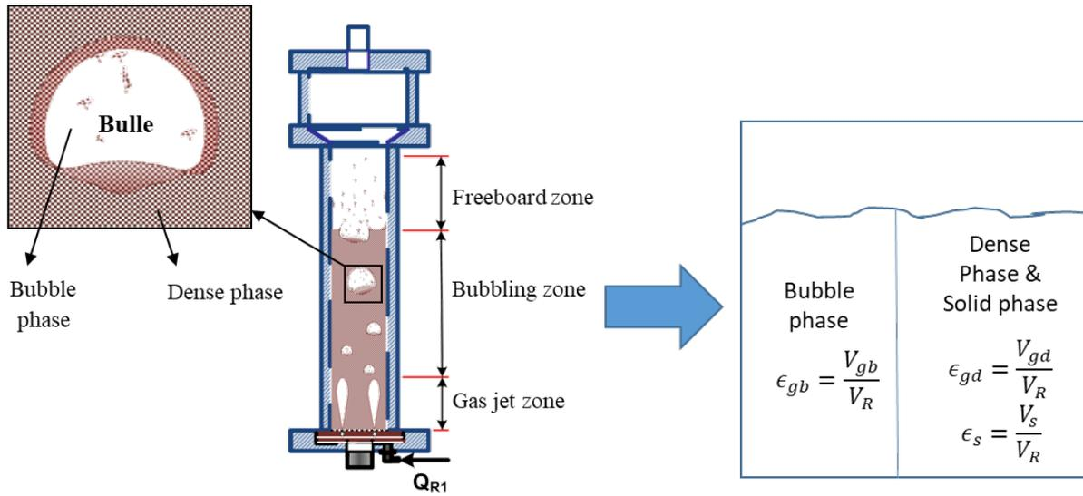
Figure 3-8: Bubbling fluidized bed two phases representation
