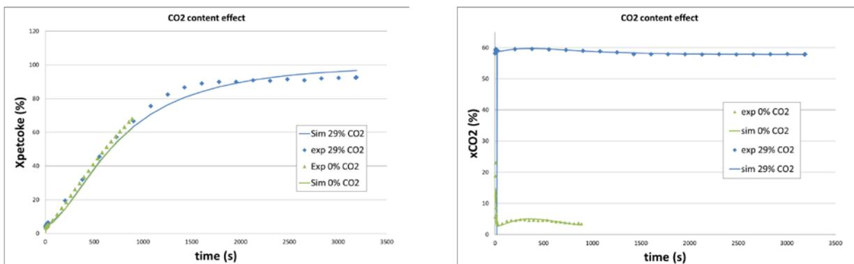
Figure 3-10: Evolution of (left) petcoke conversion and (right) carbon dioxide profiles over time at 940 °C with 50 mol% of steam diluted with 29 % or 0 % of carbon dioxide. The remaining fraction is nitrogen
