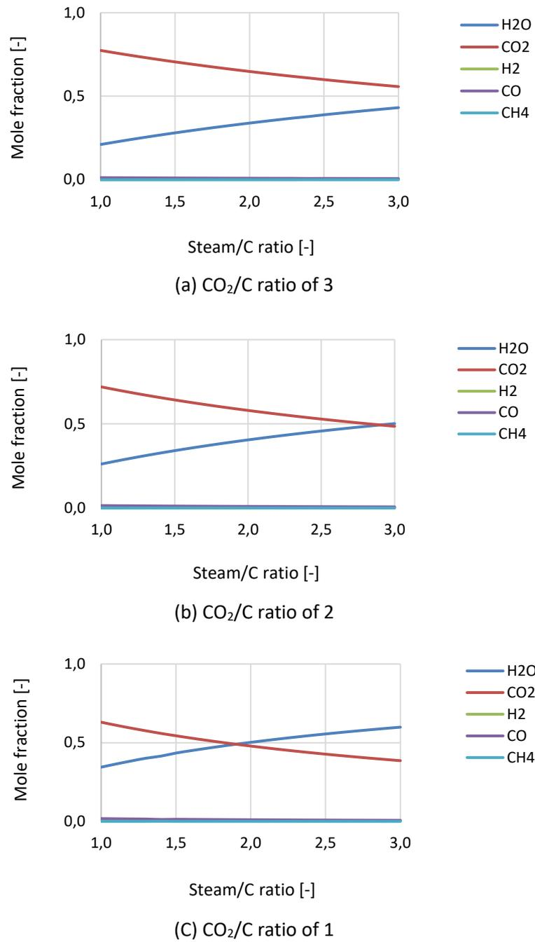
Figure 4-11 Effect of Steam/C ratio on CLC using CuO with different  $\text{CO}_2/\text{C}$  ratios at OC/C ratio of 2 and 950 °C.
