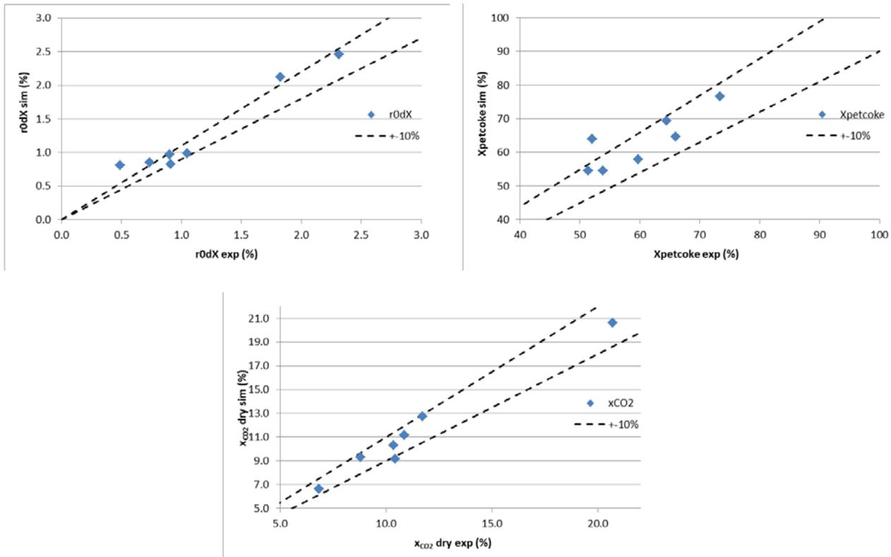
Figure 3-13: Parity diagram of r0dX,  $X_{petcoke}$  and  $x_{CO_2}$  for tests with petcoke in the 10 kW pilot modelling.
