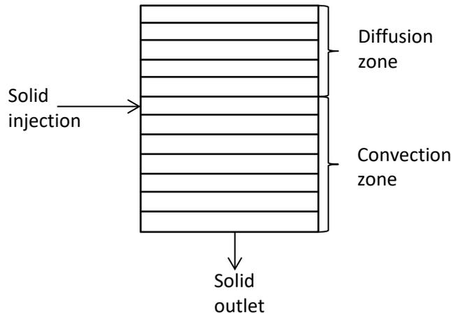
Figure 3-12: Solid circulation in the continuous fluidized bed
