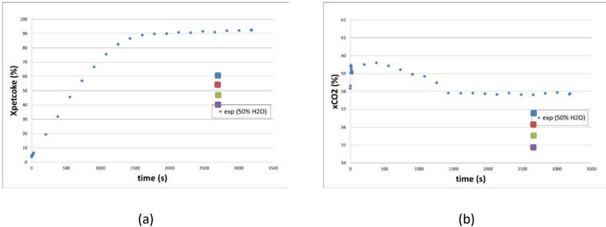
Figure 3-7: Evolution of (a)  $X_{\text{petcoke}}$  and (b) carbon dioxide outlet concentration with time for the reference steam concentration (50 mol% diluted in  $\text{CO}_2$ ) at 940 °C
