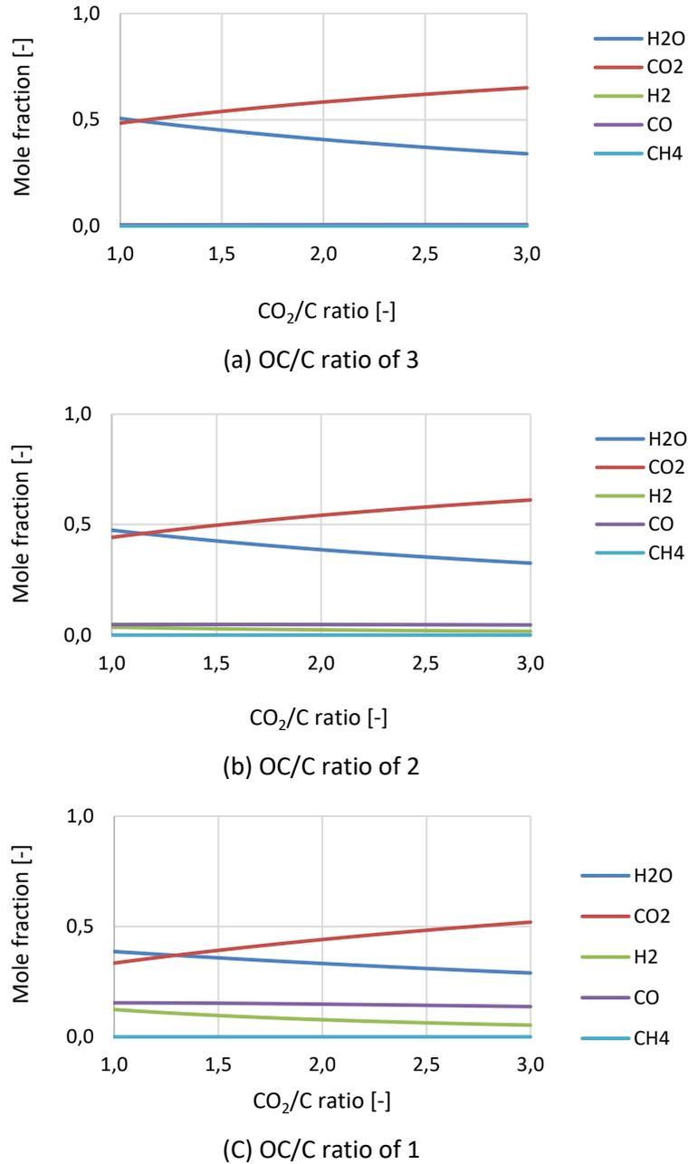
Figure 6-7 Effect of CO<sub>2</sub>/C ratio on CLC using ilmenite with different OC/C ratios at Steam/C ratio of 2 and 950 °C.
