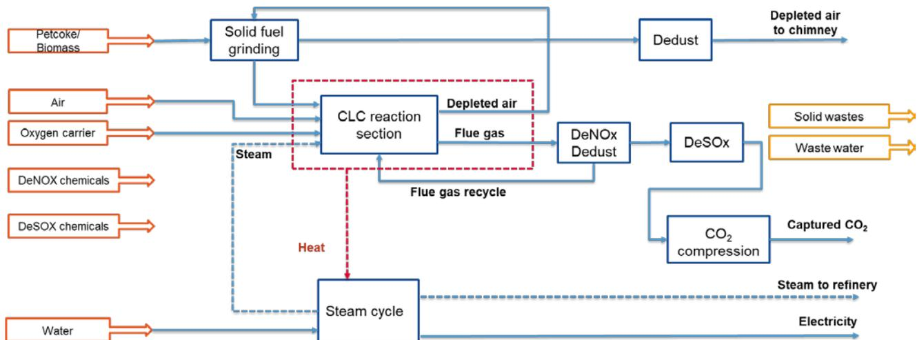
Figure 2-1: Block flow diagram of the CLC process
