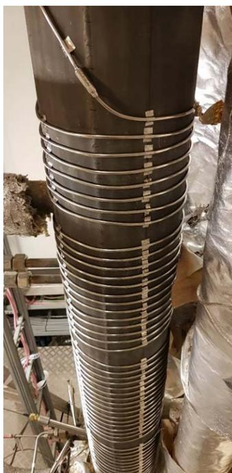
Figure A-3: Reactor heating cable
