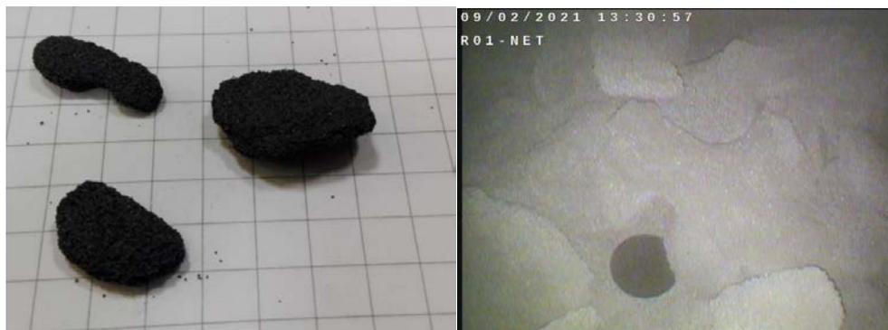
Figure 6-17: Left : agglomerates formed in the L-valve of AR2 ; right : agglomerates formed at the outlet of FR (around 5 cm of diameter)
