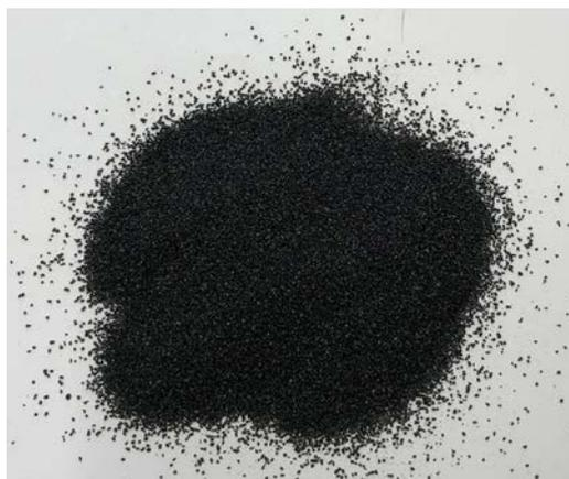
Figure 4-1: Petcoke, here shown size fraction 315 – 500  $\mu\text{m}$ .
