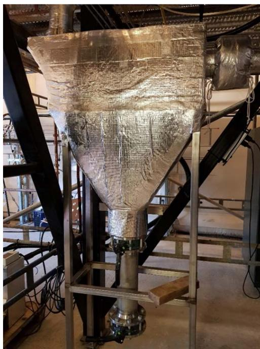
Figure A-4: Particle settling chamber
