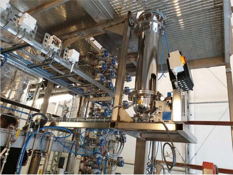
Figure A-5: Volumetric fuel feeding system
