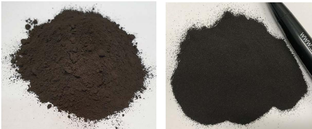
Figure 3-7: Mn-ore LY batch SINTEF ER as received (left) and after sieving (right).
