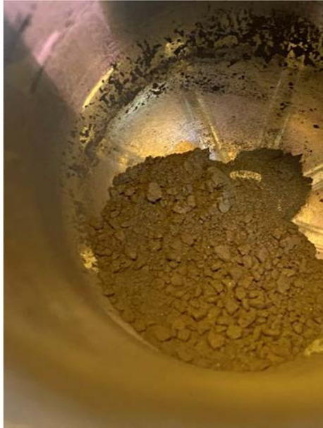
Figure 7-17: Agglomeration of LY-Mn fines in a filter.
