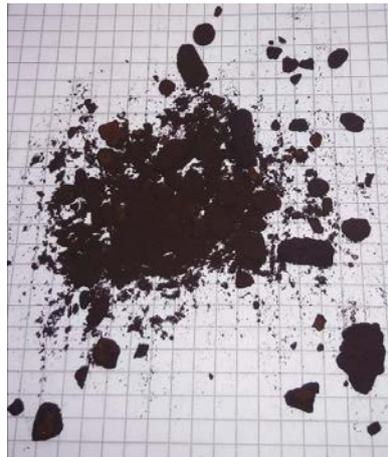
Figure 6-2: Photo of the agglomerates recovered at the end of the ageing test.
