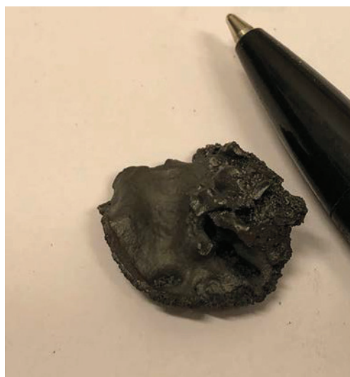
Figure 6-27: Metallic lump taken out from FR after last test with Mn-ore LY.
