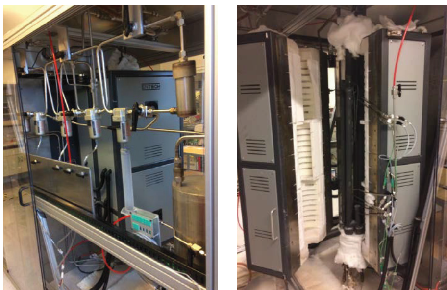
Figure 7-15: 3 kW rig with dual filter system to measure fines in filters. The system is also combined with a pressurised air system to return separated OCM back into the reactor to maintain mass circulation.
