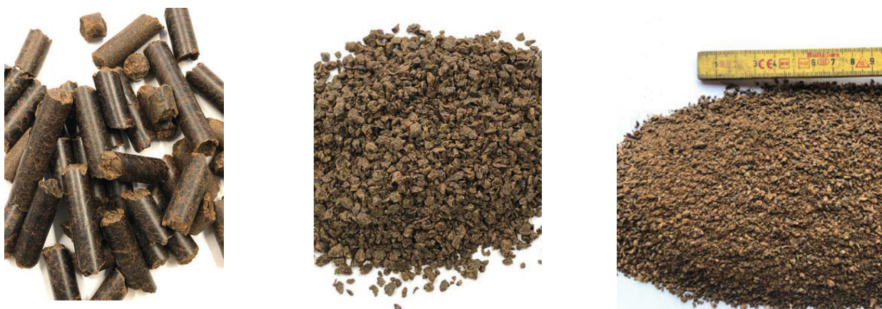
Figure 4-2: Arbaflame wood pellets. Whole (left), milled and sieved > 800 \mu\text{m} (mid), milled and un-sieved (right).
