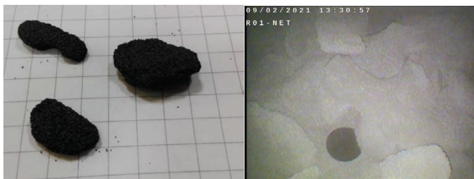
Figure 6-17: Left : agglomerates formed in the L-valve of AR2 ; right : agglomerates formed at the outlet of FR (around 5 cm of diameter)
