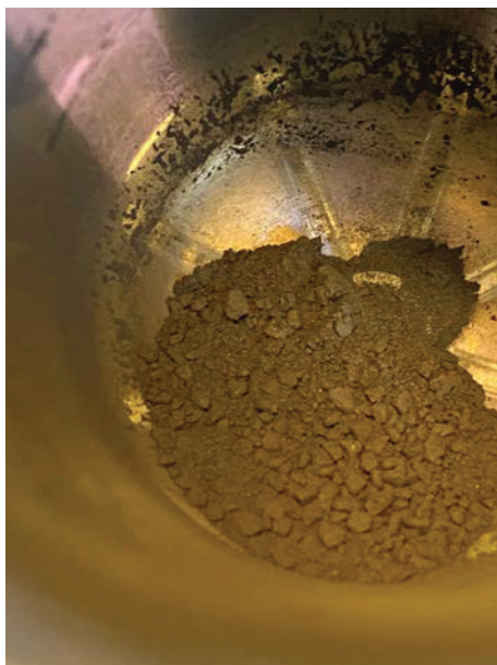
Figure 7-17: Agglomeration of LY-Mn fines in a filter.
