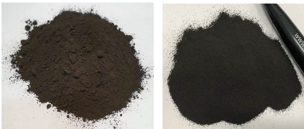
Figure 3-7: Mn-ore LY batch SINTEF ER as received (left) and after sieving (right).
