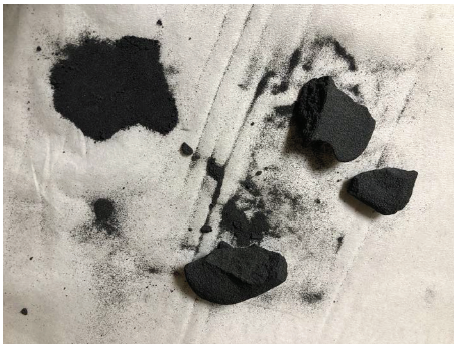
Figure 5-18: Small agglomerates taken out from reactors after agglomeration test day 2. Easily broken and crushed with the fingers.
